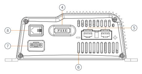
**AIR INTAKE DC OUTPUT TERMINALS** (15 2 **POWER SWITCH** 6 **AIR OUTLET** 3 **AC 240V INPUT PORT TEMPERATURE SENSOR PORT** 7 4 **OUTPUT FUSE** 8 **REMOTE (COMING SOON)**
