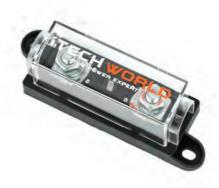
It is essential to install all recommended fuses in series within the circuit. Bolt-down fuses are the preferred choice as they guarantee a low-resistance connection. In contrast, self-resetting circuit breakers are not recommended as they may trip prematurely due to the heat generated by the current flowing through the wires.
