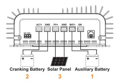
Output: connects to the battery being charged (the auxiliary battery). 1
