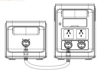
You can connect the PS1400 PR0 to a maximum of two EB1536's (sold separately), with a maximum capacity of 4608Wh, using parallel cables. Ensure that both the PS1400 PRO and the EB1536's are powered off before making the connection. Once the connection is complete, you will see "S1" and "S2" displayed on the screen.
