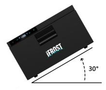
Prolonged operation with an angle of 30 degrees or more is not recommended, you should limit use in this state to a maximum of 4 hours.
